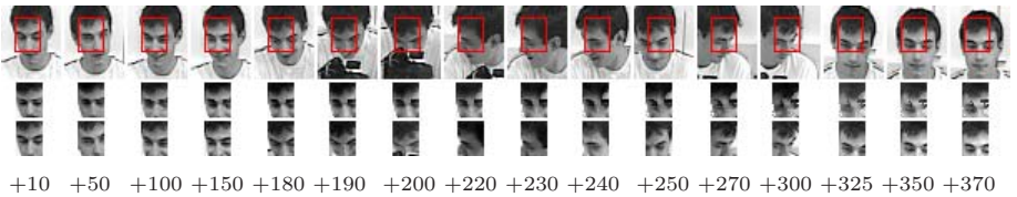
Fig. 3. Face tracking using adaptive appearance models (top row). The tracking starts at frame #11000 and the images from left to right depict some tracking results in frames #11010, #10050, etc. Next rows present the evolution of the mean of stable (middle row) and wandering (bottom row) components during tracking.
