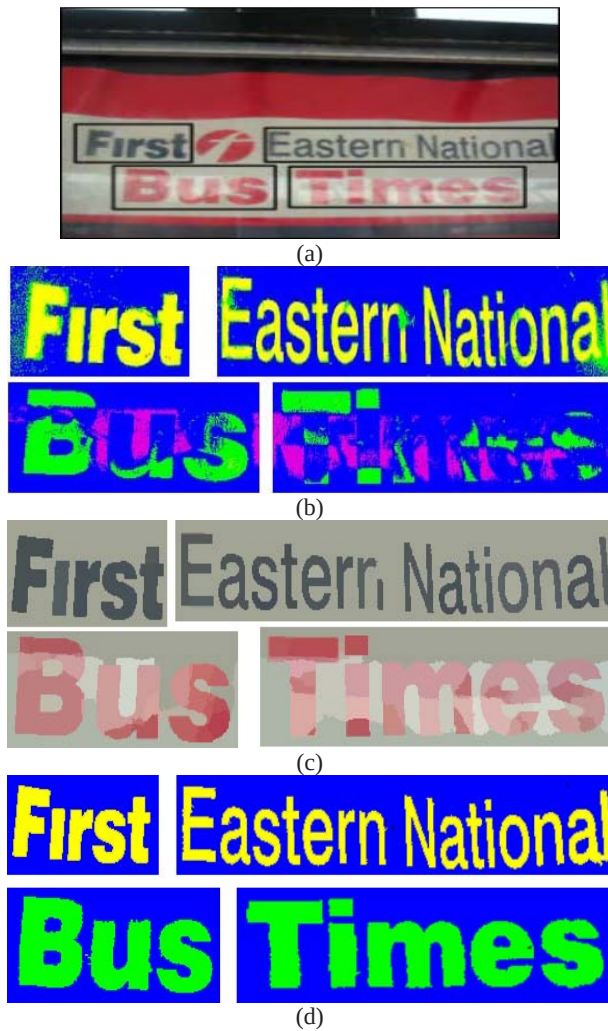
Fig. 5. The natural scene with varying intensity: (a) input image, (b) segmentation result with the I component, (c) segmentation result by proposed method, (d) segmentation result by EDISON
