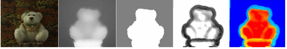
Fig. 3. A new range image R'_{12} and its reliability map. From left, input picture from C_2 , new depth map R'_{12} , depth segmentation map, reliability map, and pseudo-colored reliability map.
