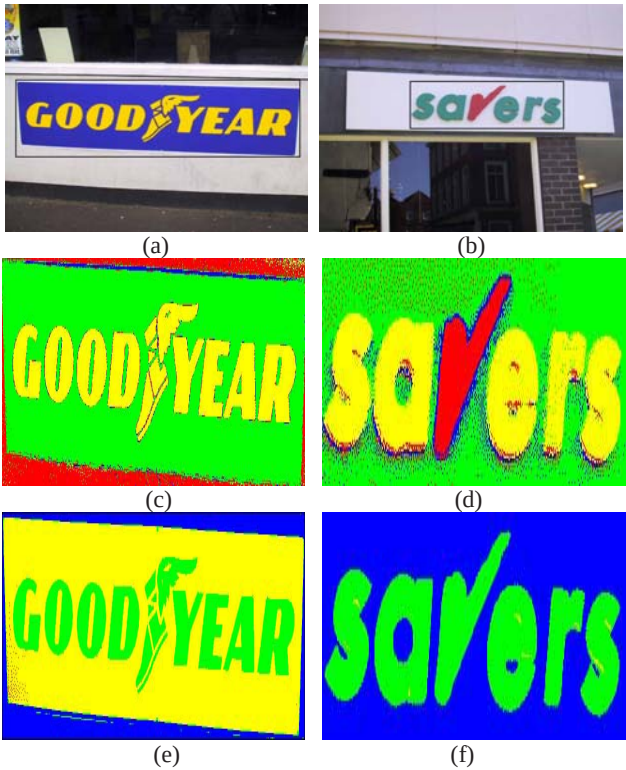
Fig. 4. The natural scene images with uniform intensity:(a) and (b) are original images, (c) and (d) are text segmentations with the H component, (e) and (f)are the results proposed method
