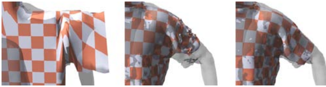
Fig. 4. On the left the initial configuration of a T-shirt template is shown. In the middle cloth particles are attracted to the closest point on the surface. On the right attraction forces are restricted to faces with similar normals.
