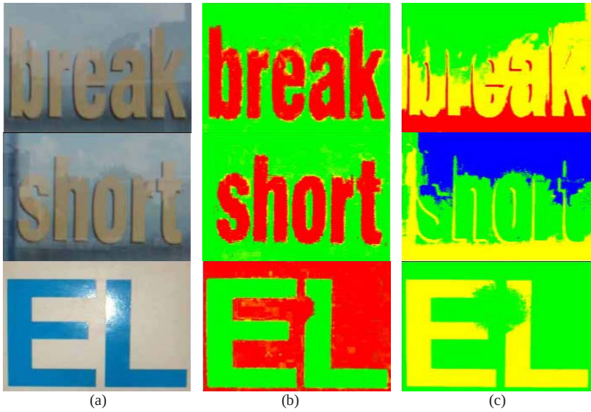
Fig. 6. Text segmentation of the images with the distortion of intensity: (a) input image, (b) proposed method, (c) intensity
